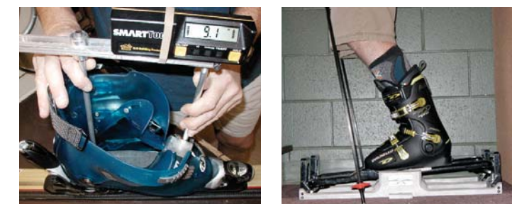
Below: ramp angle testing (left) and Campbell balancer for binding position.
